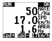
Adjust the speed value to reflect a typical working speed & press the RUN button to take the Jackal off Hold
